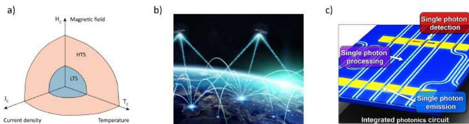
Figure 5.1: a) Schematic phase diagram of the superconducting phase in low-temperature superconductors (LTS) and high-temperature superconductors (HTS). b) Illustration of high-speed optical communications. Credit: TELESAT. c) Concept for on-chip photonics in a planar waveguide platform. Credit: R.J. Shiue and D. Englund.
