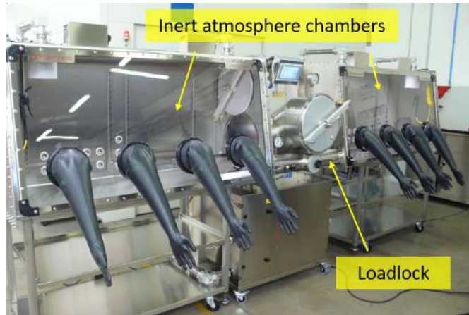
Figure 2.6: General view of the Jacomex glovebox system.
