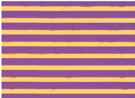
Figure 5.9: Non-detrimental residuals of the photoresist film near the edges of the metal layer. Although they are visually unpleasing and can be mistaken for breaks in the contacts, this cosmetic defect does not impact the functionality of the device, as all contacts are electrically intact.
